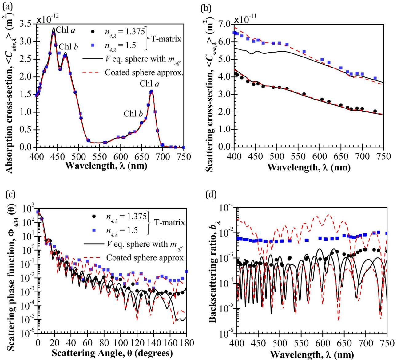
**Fig. 3.** Comparison between the estimated spectral (a) absorption cross section ( $C_{abs,\lambda}$ ), (b) scattering cross section ( $C_{sca,\lambda}$ ), (c) scattering phase function  $\Phi_{634}(\theta)$  at wavelength 634 nm, and (d) spectral backscattering ratio  $b_\lambda$  of heterogeneous eukaryotic microalgal cells with wall refractive indices  $n_{4,\lambda} = 1.375$  and  $1.5$  and those from homogeneous and coated sphere approximations.
